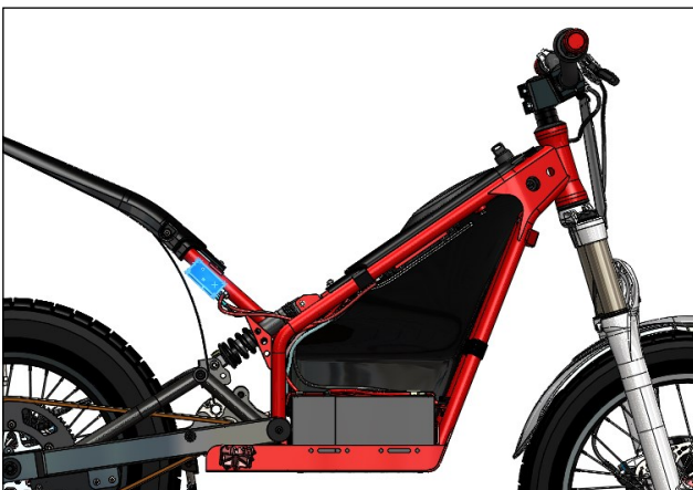
Image 4a - Previous relay mounting position.
