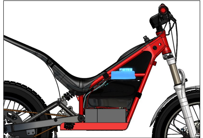
Image 3b—Relocated controller & fuse holder.
