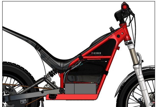
Image 2b - Controller cover removed on a 2017 model.
