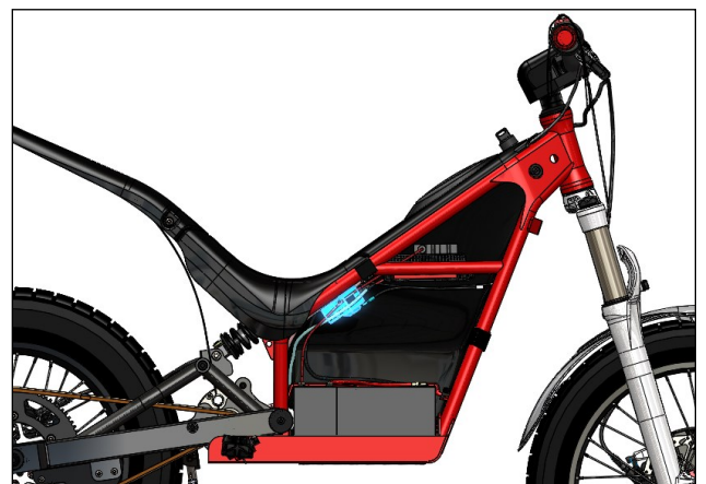
Image 4b - New relay location on 2017+ frames.
