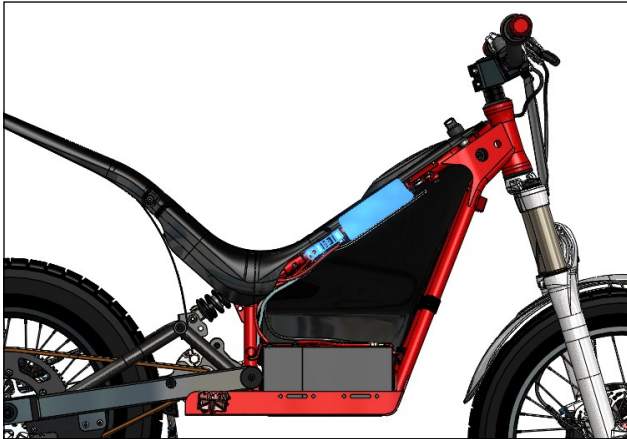
Image 3a - Previous controller & fuse holder positions.
