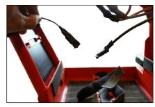
The bike will run perfectly OK with the sensor disconnected, we suggest you send the motor serial number to info@osetbikes.com so it is recorded.
