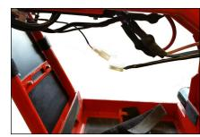
4. Seal both connecters with something suitable, such as heat shrink and cable tie out of the way.
