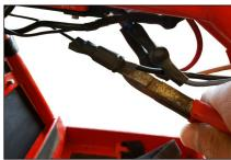
3. Disconnect the thermal sensor
