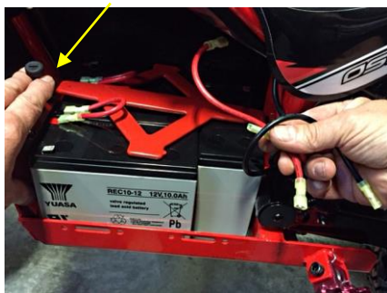
Battery strap fixing bolt
